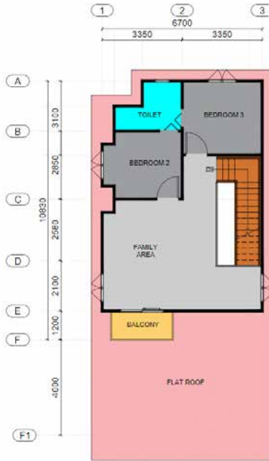
MyIOS Single House 2-storey P12 First Floor Plan Layout
