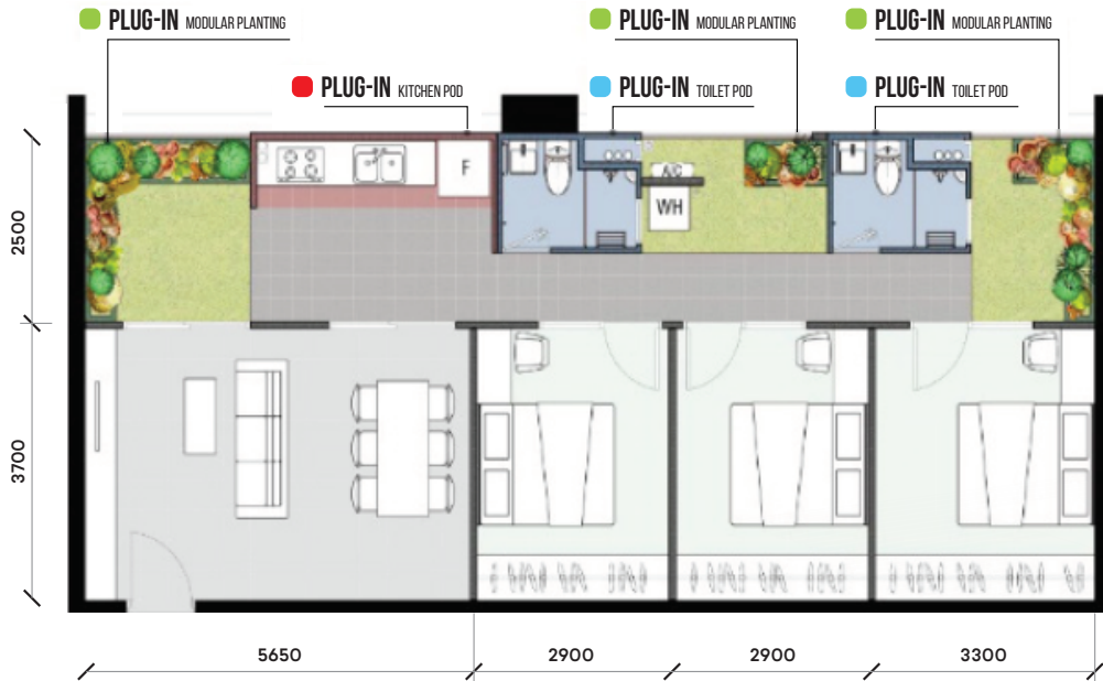
Example of open plan design concept where internal wall between bedrooms can be removed or adjusted and components such as bathroom can be plugged-in
