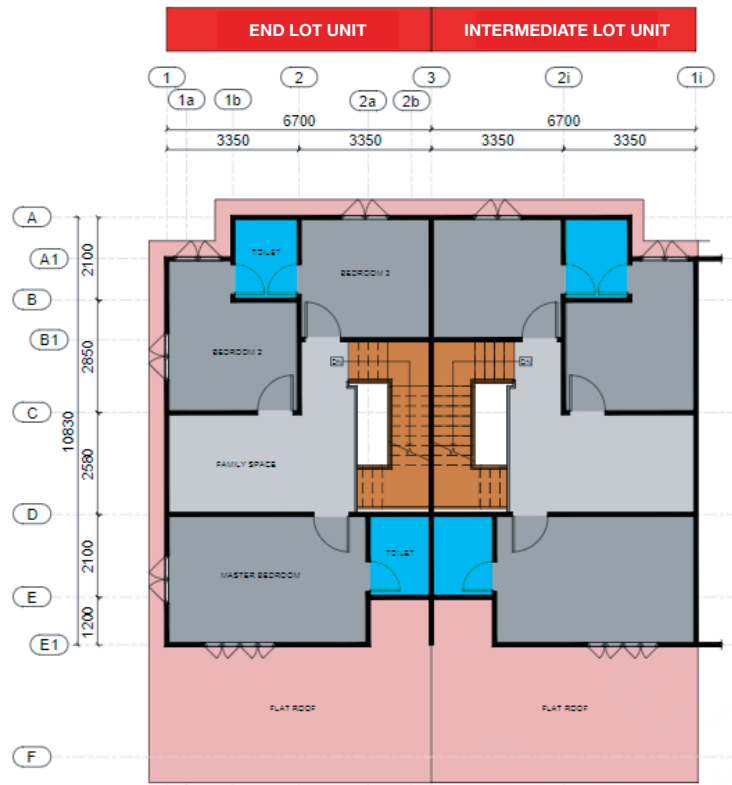
MyIOS Terrace House 2-storey P07 First Floor Plan Layout
