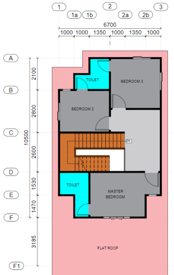
MyIOS Single House 2-storey P13 First Floor Plan Layout
